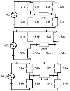
Fig3: Modes of operation Matrix converter.
