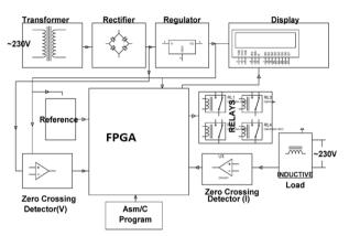
Fig2: Power Factor Correction using FPGA.
